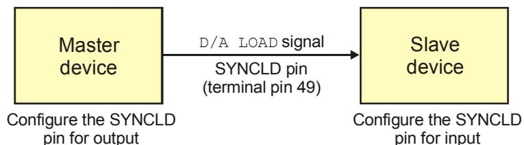
Figure 8. Synchronizing the update of multiple devices
