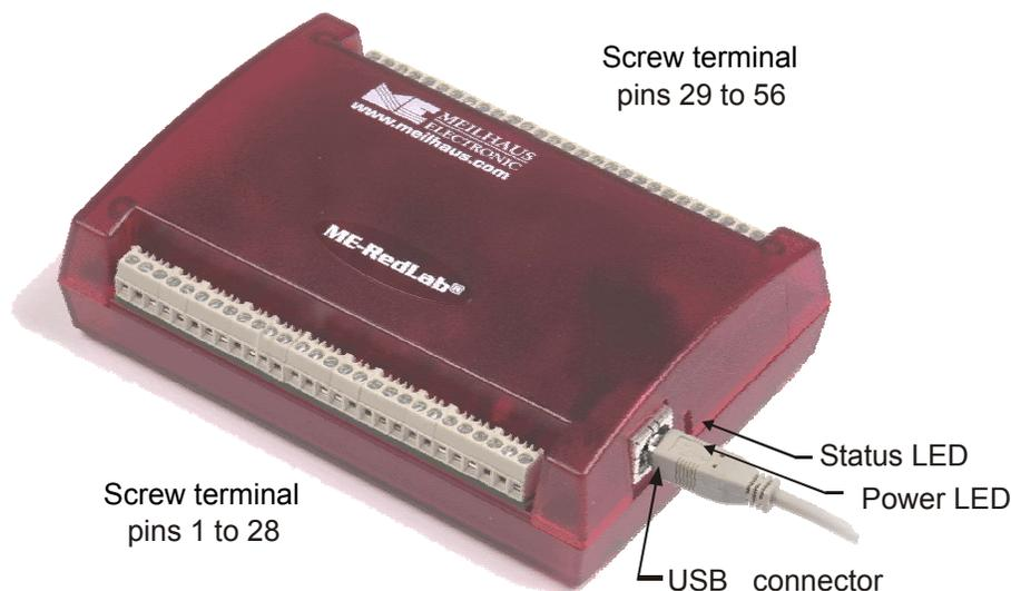
Figure 3. RedLab 3105 external components
