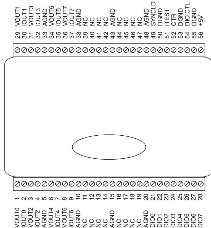
Figure 5. RedLab 3104 signal pin out
