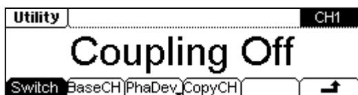
**Channel Coupling:** Once you setup the base channel and the Frequency/Phase deviation of the two channels, the Frequency/Phase of the other one will vary with the base channel and will still keep the deviation you have selected.
