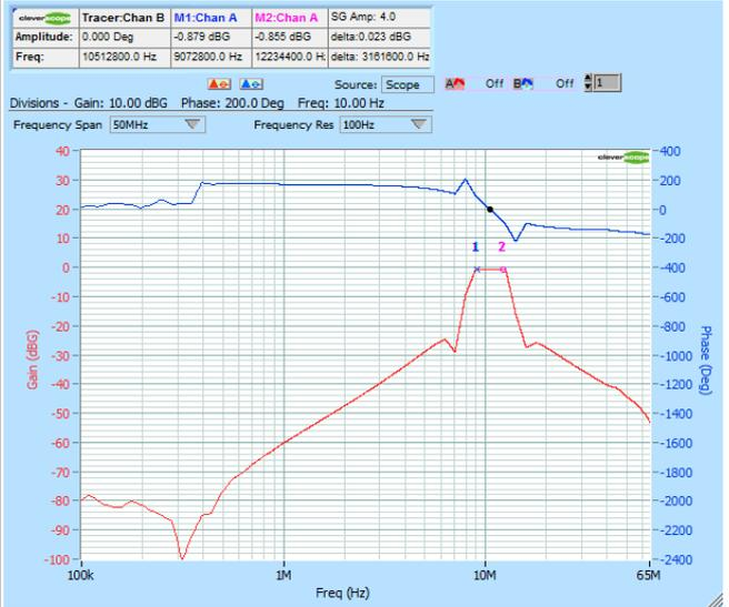
**TLV70433 PSRR using CS1070 (1A 50 MHz op-amp):**
