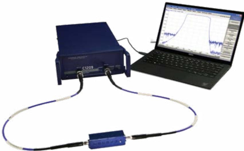
Cobalt 20 GHz VNAs have 135 dB dynamic range at 1 Hz IFBW, which allows them to maintain a wide measurement range at high measurement speeds. Measurement of all S-parameters of a BTS filter with full two-port and 801 measurement points with 1 MHz IFBW takes only 17.5ms while maintaining a measurement range of over 85 dB. This time is almost completely determined by the IFBW of the VNA. This measurement speed allows for real time tuning of high isolation BTS filters.
