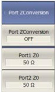
This function converts the S-parameters measured at a 50 Ω port into values which would be seen if measured at a test port with arbitrary impedance.
