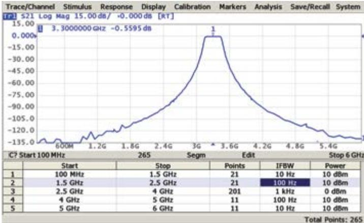
The VNA has a large frequency range with the option of frequency scan segmentation. This allows for optimal use of the instrument to realize maximum dynamic range while maintaining high measurement speed.
