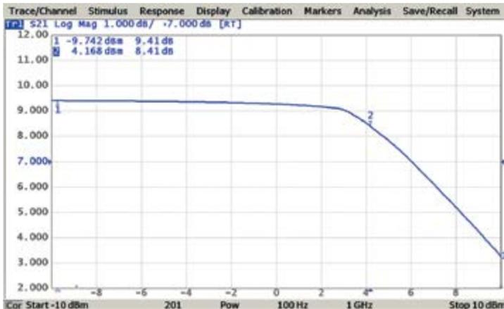
The power sweep feature turns compression point recognition, one of the most fundamental and complex amplifier measurements, into a simple and accurate operation.
