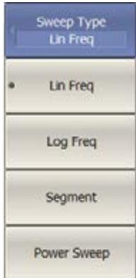
**Sweep type:** Linear frequency sweep and logarithmic frequency sweep are performed with fixed output power. Linear power sweep is a fixed frequency.
