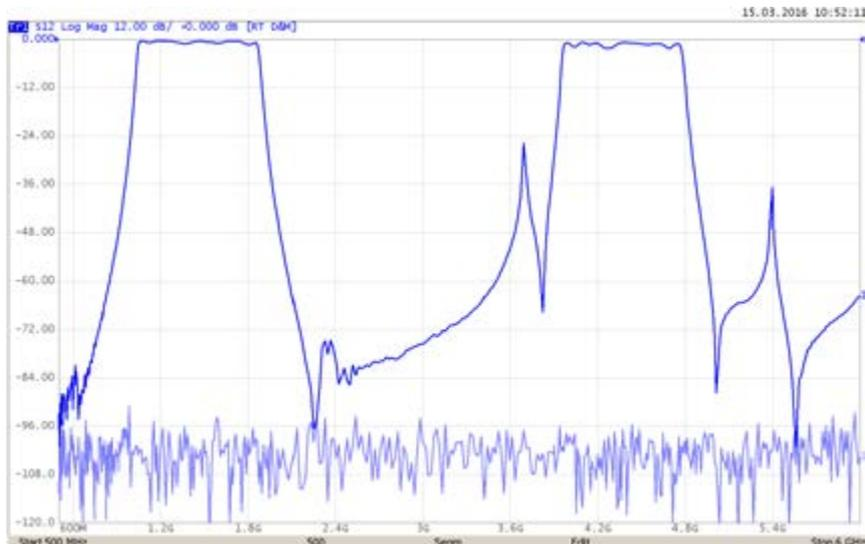
The 135 dB dynamic range of Cobalt VNAs combined with high measurement speed per point allows measurement of SAW filters' S-parameters with full 2-port calibration and 1601 measurement points in less than 32 ms while still maintaining more than 85 dB measurement range (IFBW at 1 MHz). This measurement speed corresponds to the performance of the most advanced handlers used for automatic verification of mass-produced SAW filters.
