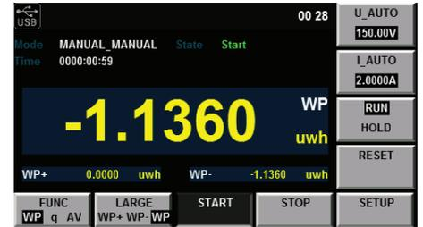
The integration function is useful for analyzing bought and sold electrical energy of a grid tied power systems. The 5335C meter provides current integral and active power integral (Wh) functionality using automatic range switching for accurate measurement results.
